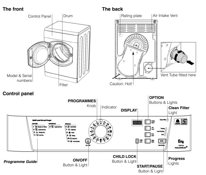
The **ON/OFF** button/light **()**: If the dryer is running and this button is pressed, the dryer is turned off. Press again, the dryer restarts. The light signals that your dryer is in use or ready to select a programme.
